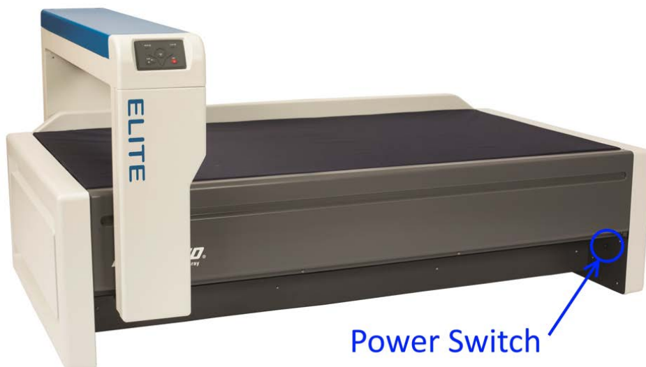
Figure 4-16: Power Switch location
